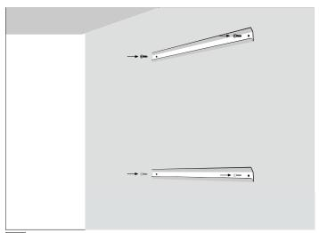
Plan where you're going to install your TV. Mark the wall where your brackets would be mounted, then drill holes into it. Screw the two mounts onto the wall.
