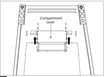
Remove the Compartment Cover Remove the protective cover from the compartment.
