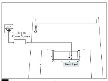
**Plug the Power Cord**Connect the power supply to the power input port located at the back of the TV and plug the other end to your power source.
