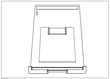
4 Lay the Mirror on Flat Padded Surface Lay the mirror down on a flat, soft surface to avoid damages or scratches.
